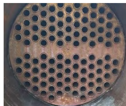
North Side of HEX Before & After Cleaning
